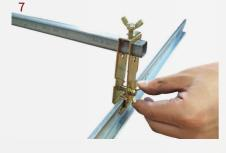
Tighten the wing nut to a torque of 3 ft-lbs / 4 N\*m to secure end brackets to the rails.
